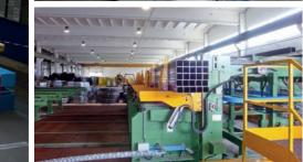
FIMI tube packers are completely smart systems which allow the preparation of square, rectangular and hexagonal bundles.
