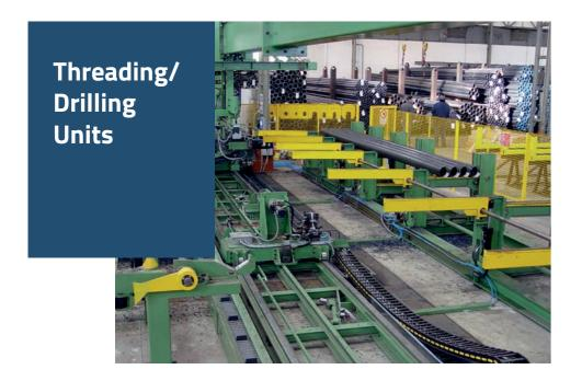
The threading unit is used to rework the ends of the tube to create an internal or external thread defined by a specific product.
